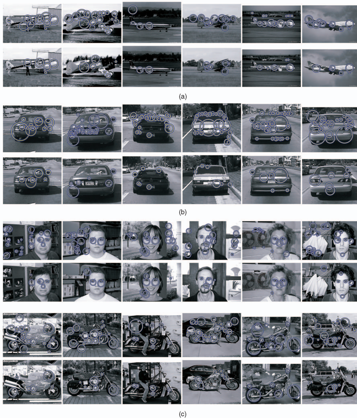
Fig. 7. Sample test images that are classified as containing a targeted object. For each block of images, images in the first row show all the detected salient regions enclosed by circles, and the corresponding images in the second row show only the regions that are identified by MILES as parts of the object. (a) Airplanes, (b) cars, (c) faces, and (d) motorbikes.
